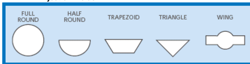
Figure 27. Schematic showing typical runner designs found in injection molds
